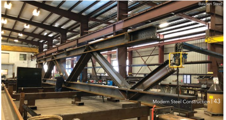
above and below: The trusses exceeded project fabricator Basden Steel's crane capacity of 27 tons, so the shop developed custom jacking systems to maneuver each truss.
